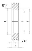
Installation direction: o-ring sits on chamfer.
